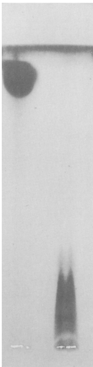
FIG. 2. Thin layer chromatogram of purified final product: left lane starting ceramide galactoside; right lane purified ceramide galacturonate.
