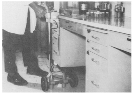
FIG. 3. Floor monitor for ^{14}\text{C} .
