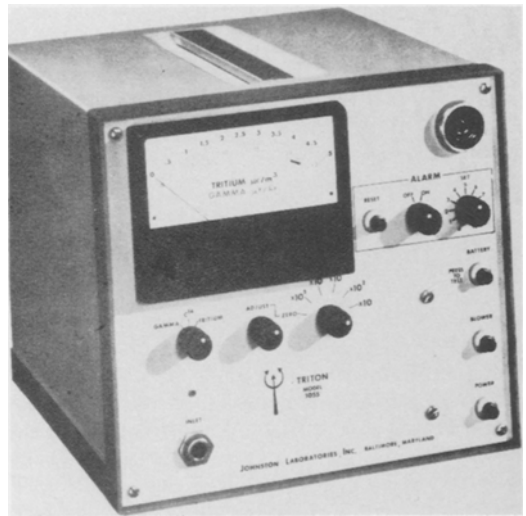
FIG. 4. Flow-through ionization chamber for monitoring concentration of airborne 3 H and 14 C (Courtesy of Johnson Laboratories, Inc.).
